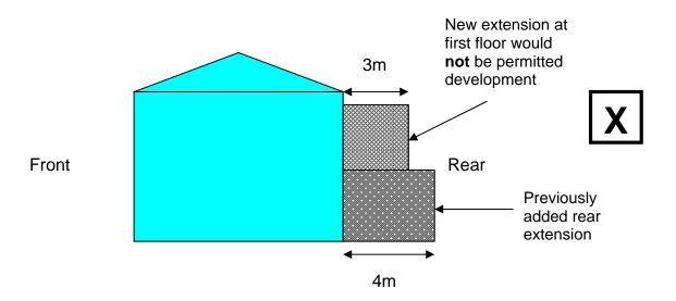
In addition, where the extension or enlarged part of the house has more than one storey, it must be a minimum of seven metres away from the boundary of the land surrounding any house opposite. For example:
