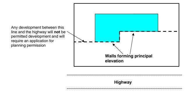
If a house lies on a corner plot where a side elevation also fronts a highway, there will be an additional restriction on permitted development to the side of the house:
