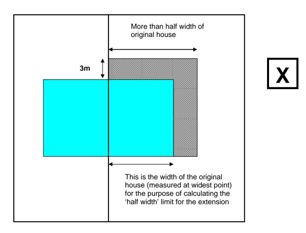
In some situations, it may be that permitted development is undertaken in separate stages, for example, a side extension may be built first, and then a rear extension added at a later date. For example:
