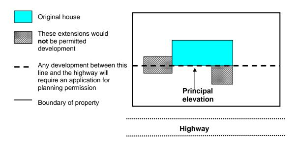
The principal elevation could include more than one wall facing in the same direction - for example, where there are large bay windows on the front elevation, or where there is an 'L' shaped frontage. In such cases, all such walls will form the principal elevation and the line for determining what constitutes 'extends beyond a wall' will follow these walls.
