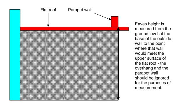
Where the existing house has eaves of different heights, then the restriction on the height of the eaves for the part of the house enlarged, improved or altered is measured against the highest level of eaves on the existing house. However, where a house is built on sloping ground, the height of the eaves on the existing house should be measured in terms of the elevation from which any extension of a house is to be made.
