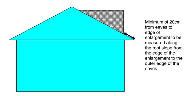
This 20cm set back will be required unless it can be demonstrated that this is not possible due to practical or structural considerations. One circumstance where it will not prove practical to maintain this 20cm distance will be where a dormer on a side extension of a house joins an existing, or proposed, dormer on the main roof of the house.
