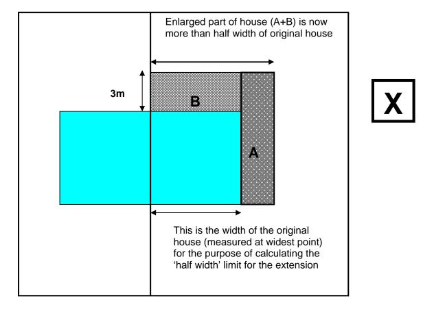
In the example above, if the side extension (**A**) was built first, it would meet the requirement for being no more than half of the width of the original house. However, the later addition of the rear extension (**B**) would mean that the total width would be more than half the width of the house. The rear extension would therefore require an application for planning permission.
