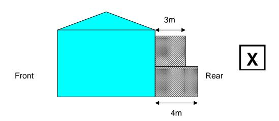
Similarly, if a *detached* house has an existing, single storey, ground floor extension that was not part of the original house and which extended beyond the rear wall by more than three metres, then it would not be possible to add an additional first floor extension above this without an application for planning permission - because the enlarged part of the house would then consist of more than one storey and would extend beyond a rear wall by more than three metres:
