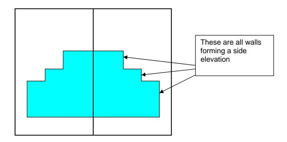
Where an extension is beyond **any** side wall, the restrictions in **(h)** will apply. Any extension can only be a single storey, is limited to four metres in height and can only be half the width of the original house. The width of the original house should be calculated at its widest point.
