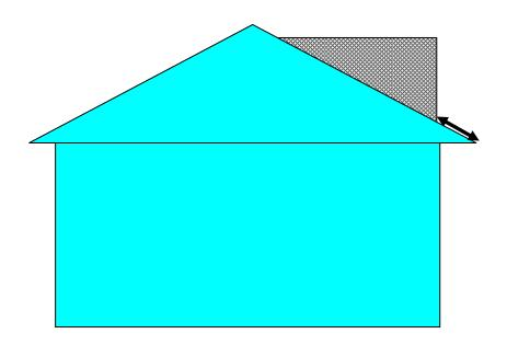
Minimum of 20cm from eaves to edge of enlargement to be measured along the roof slope from the edge of the enlargement to the outer edge of the eaves
