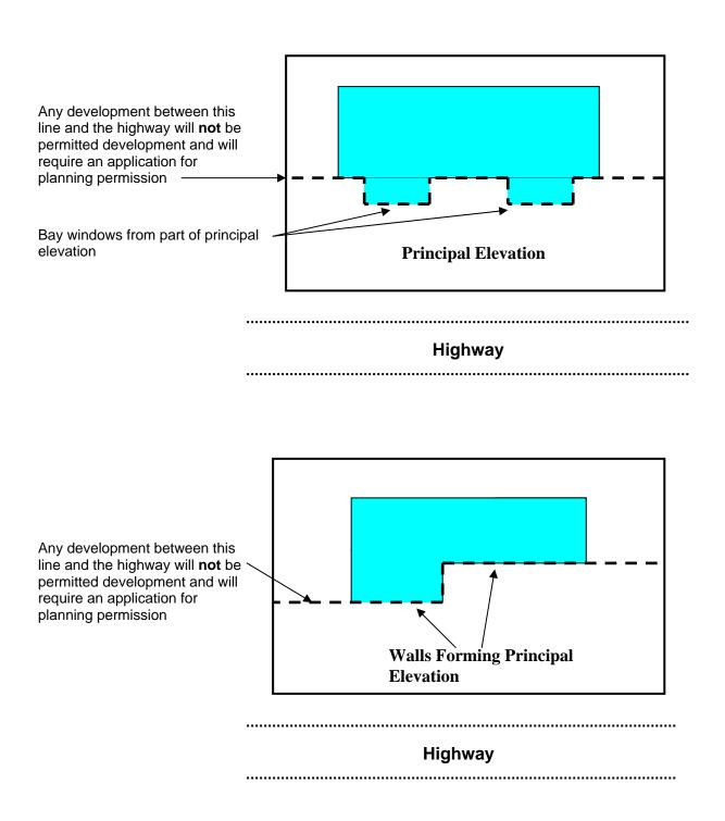
If a house lies on a corner plot where a side elevation also fronts a highway, there will be an additional restriction on permitted development to the side of the house:
