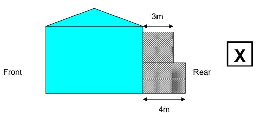
Similarly, if a *detached* house has an existing, single storey, ground floor extension that was not part of the original house and which extended beyond the rear wall by more than 3 metres, then it would not be possible to add an additional first floor extension above this without an application for planning permission - because the enlarged part of the house would then consist of more than one storey and would extend beyond a rear wall by more than 3 metres:
