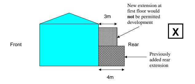
In addition, where the extension or enlarged part of the house has more than one storey, it must be a minimum of 7 metres away from the boundary of the land surrounding any house opposite. For example:
