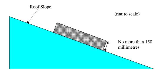
This limitation to projection from the roof plane should not be applied in cases where the roof of an extension to a house that is permitted development under Class A is joined to the roof of the original house. In such cases, the roof of the extension should not be considered as protruding from the original roof.
