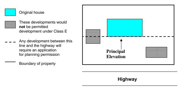
Where the principal elevation comprises more than one wall facing in the same direction, all such walls will form part of the principal elevation and the line for determining what constitutes "extends beyond a wall" will follow these walls:
