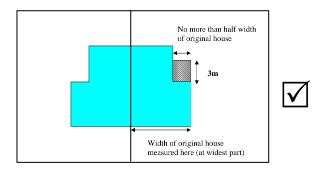
In the following example, although the extension is less than half the width of the original house and extends beyond the rear wall at '**A**" by only 3 metres, it extends beyond the rear wall '**B**' by more than 3 metres. It would therefore **not** be permitted development and will require an application for planning permission.
