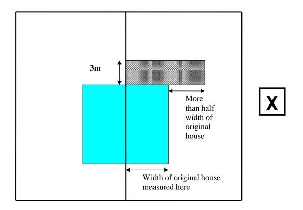
Although in this example, the extension only extends 3 metres beyond the rear wall, that part that extends beyond a side wall has a width of more than half the width of the original house. An application for planning permission would therefore be required.
