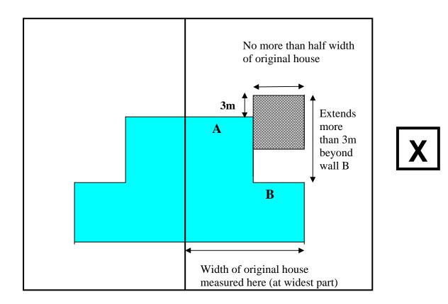
In other cases, an extension may comprise both elements of a rear and side extension. Examples could include:
