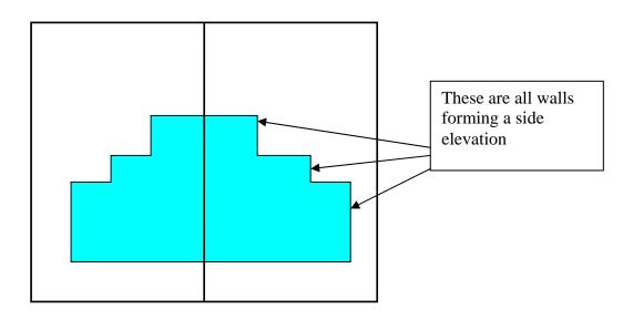
Where an extension is beyond **any** side wall, the restrictions in **(h)** will apply. Any extension can only be a single storey, is limited to 4 metres in height and can only be half the width of the original house. The width of the original house should be calculated at its widest point.
