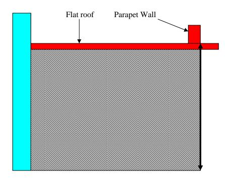
Eaves height is measured from the ground level at the base of the outside wall to the point where that wall would meet the upper surface of the flat roof - the overhang and the parapet wall should be ignored for the purposes of measurement.
