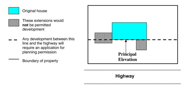
The principal elevation could include more than one wall facing in the same direction - for example, where there are large bay windows on the front elevation, or where there is an 'L' shaped frontage. In such cases, all such walls will form the principal elevation and the line for determining what constitutes "extends beyond a wall" will follow these walls.
